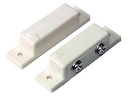
This type of Proximity Reed Switch and paired magnet is usually a Normally Closed (NC) type. They include a mounting flange and are often used as door sensors. They can be purchased from electronic stores and many hardware stores. These switches are inexpensive and work well as a dyno speed sensor. You can swap the magnet for a small Rare Earth magnet which may be easier to mount on a dyno shaft.
